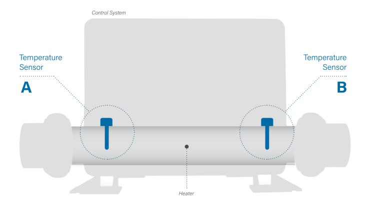
Follow this sequence to view separate temperature readings from sensor A and sensor B on the Main screen.
